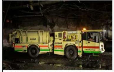
Each of the Normet SmartDrive EVs are based on a modular Battery Electric Vehicle
