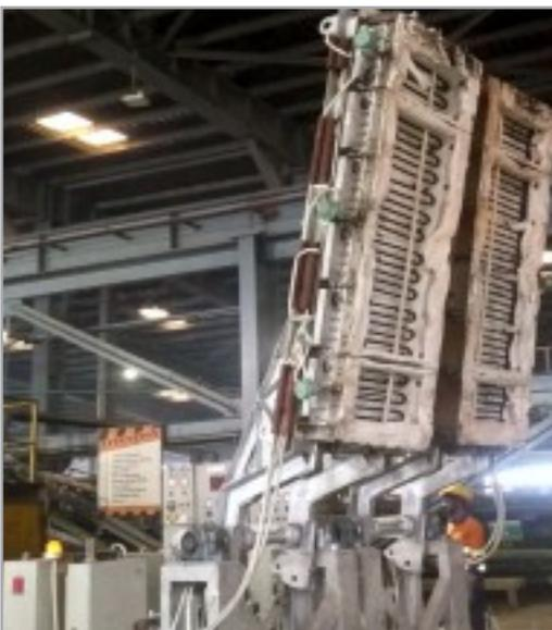
During Jumbo casting there is requirement of mould heaters for proper physical quality finish of Jumbo Jumbo ingots. For that, Push-Pull type Electric mould top heaters. New electric top heaters with pneumatic lifting mechanism have been installed to reduce the Electrical & ergonomic hazard in Jumbo casting area as compared to Push-Pull type Mould top heaters.
