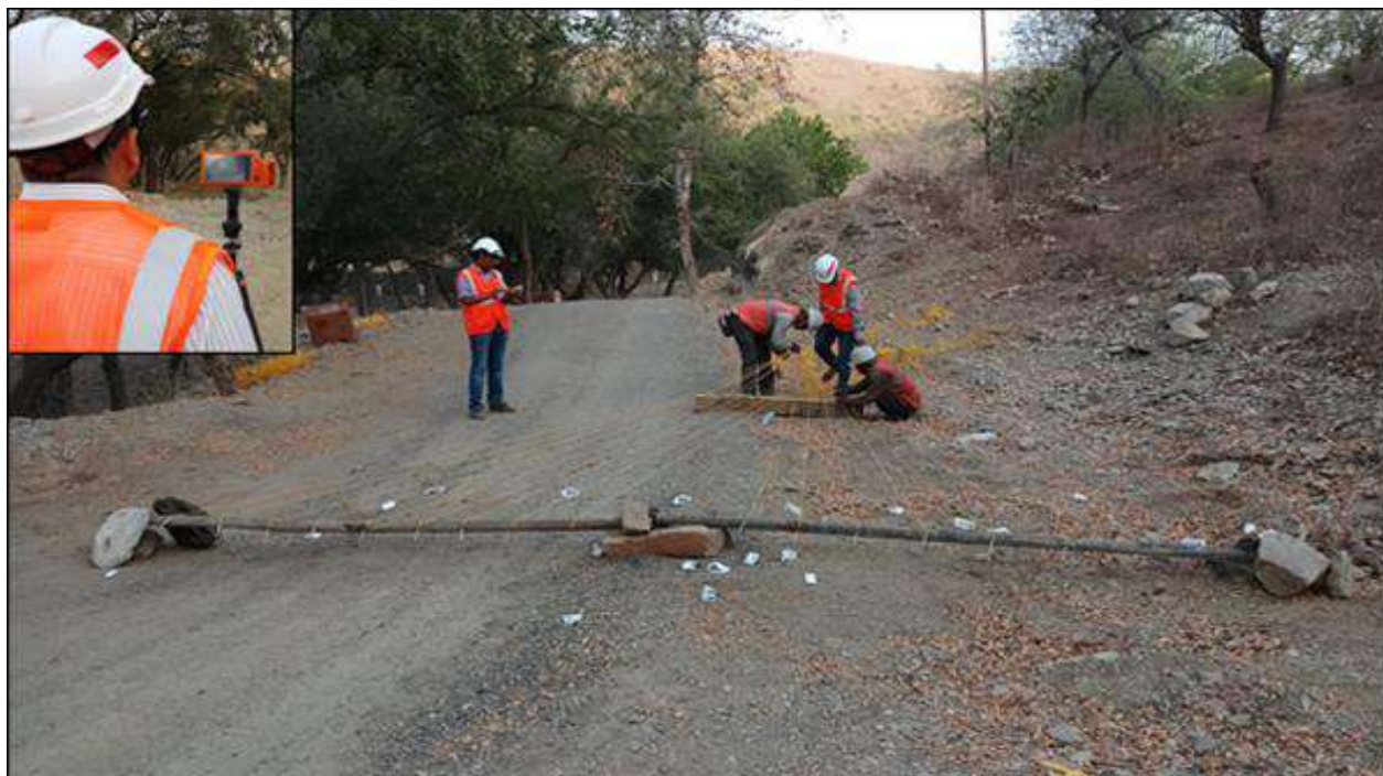
Photograph 2. View of NONEL delay detonators (3 sets of delay number 1-5) connection for delay detonator scattering test.
