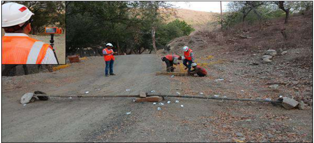
Photograph 2. View of NONEL delay detonators (3 sets of delay number 1-5) connection for delay detonator scattering test.
