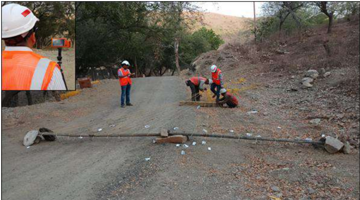
Photograph 5. View of NONEL delay detonators (3 sets of delay number 1-5) connection for delay detonator scattering test.
