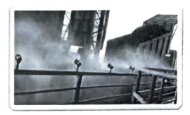
4. Dust suppression through water sprinkling on haul road at surface and in underground
