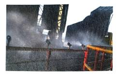
4. Dust suppression through water sprinkling on haul road at surface and in underground
