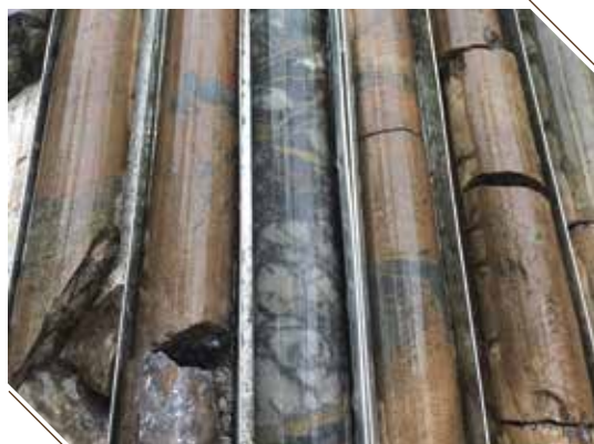
High grade mineralisation (zinc & lead) intersected in exploration drill hole
