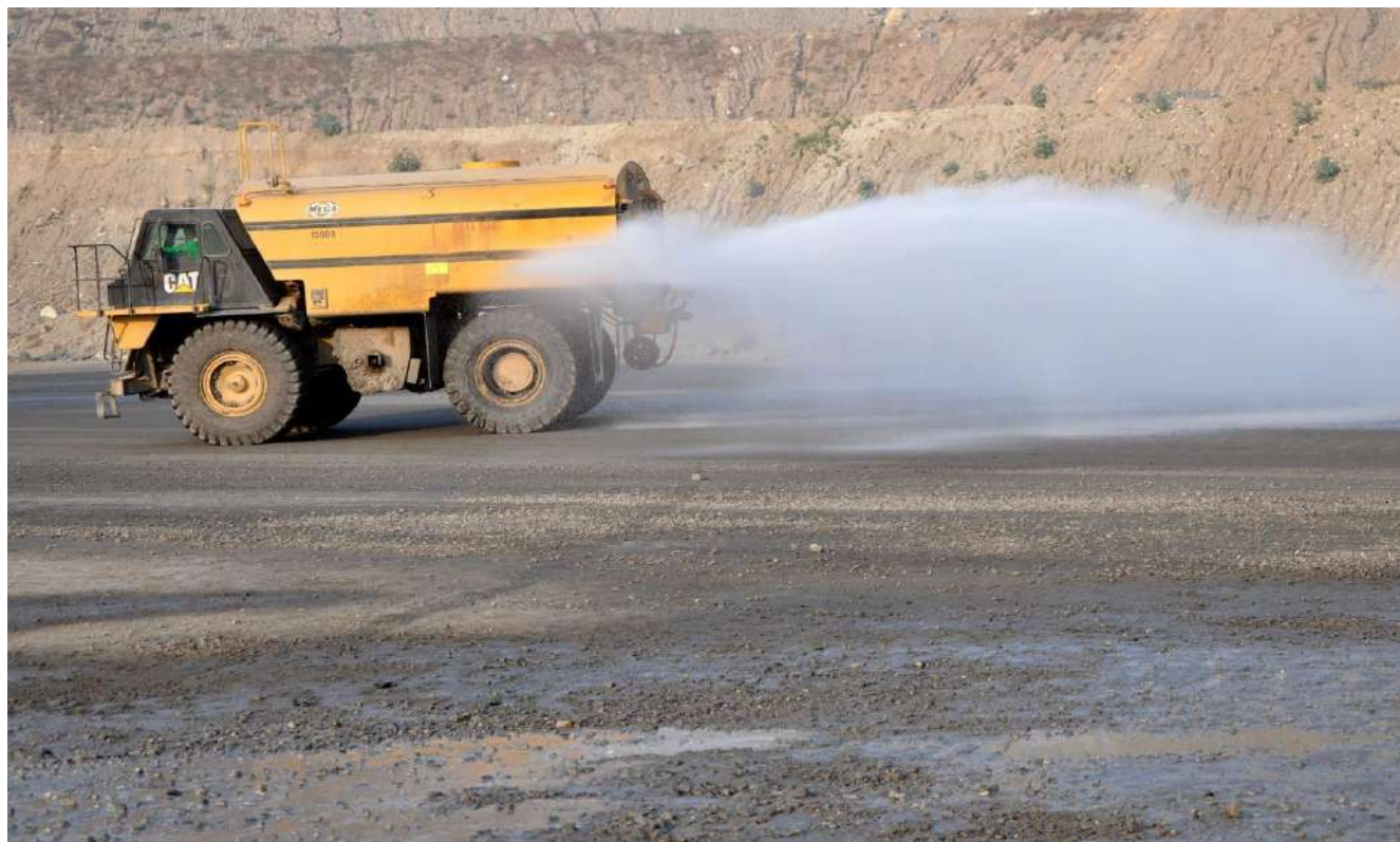
40KL Water sprinkler
