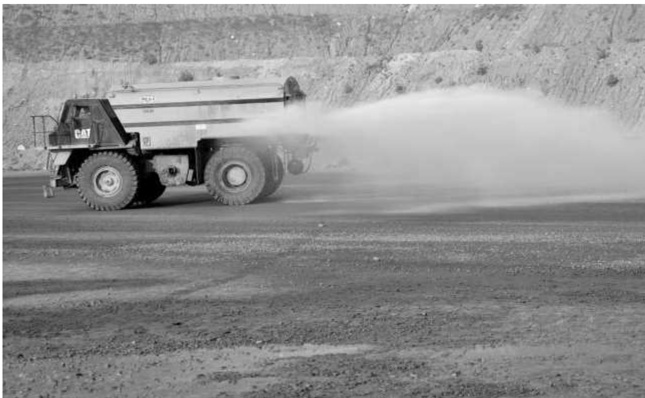
40KL Water sprinkler
