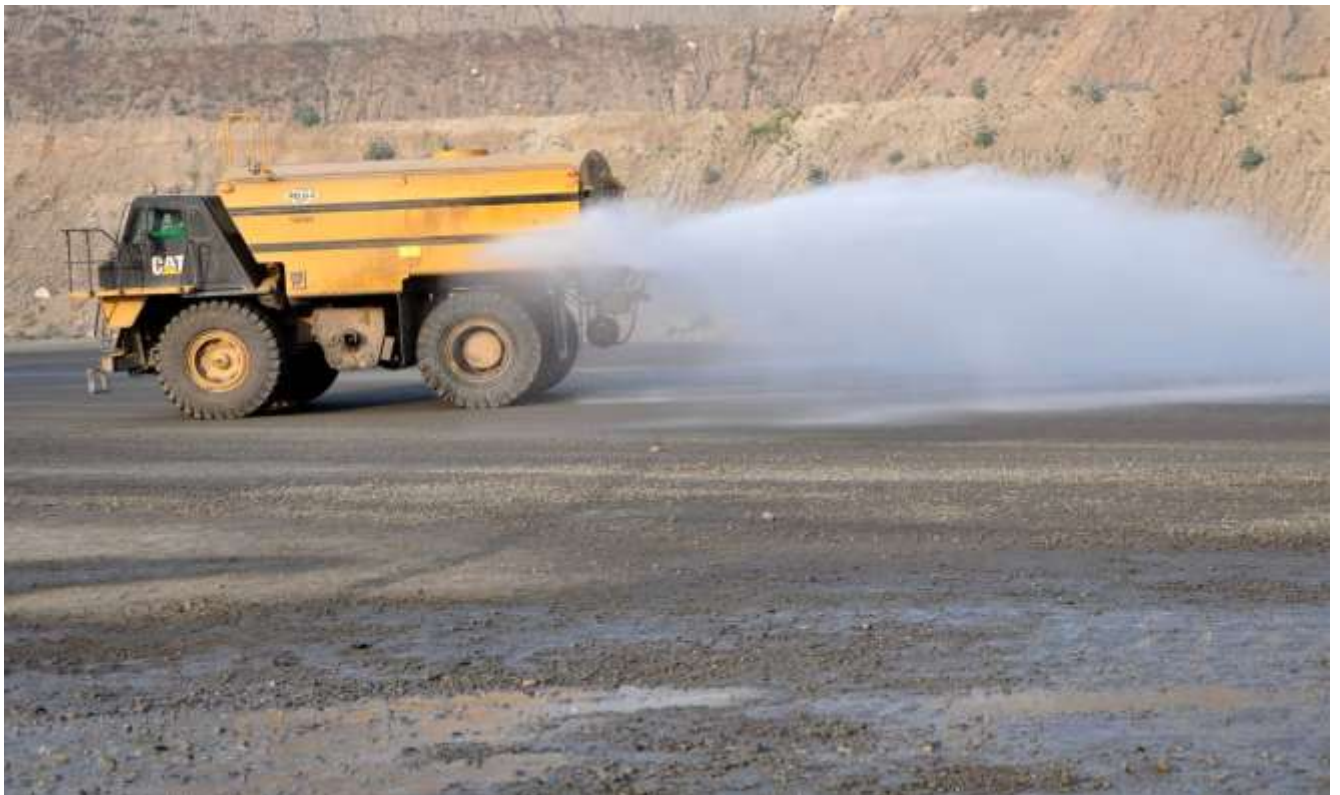
40KL Water sprinkler
