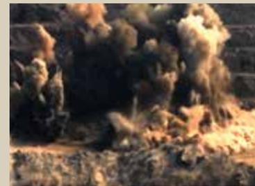
Successful firing with combined production and trim blast at Rampura open cast
