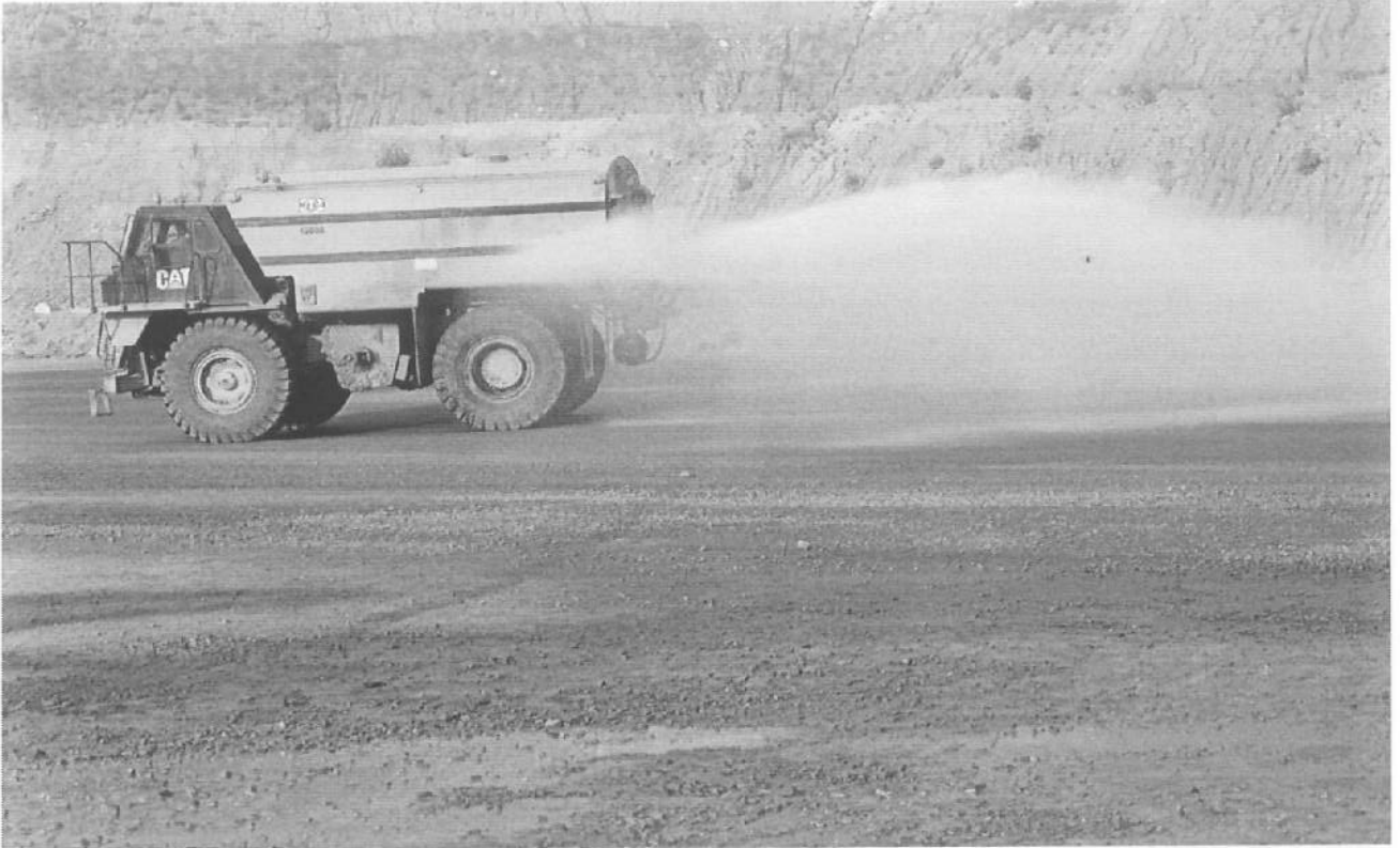
40KL Water sprinkler
