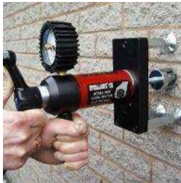
Figure29: AnAnchorTesting Devicehelpsinensuring whethertheinstalledanchors areadequateornot
