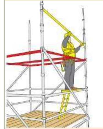
Figure 66: Scaffolders installing a guardrail in advance to the next lift from a scaffolders' step protected by the ledgers and transoms
