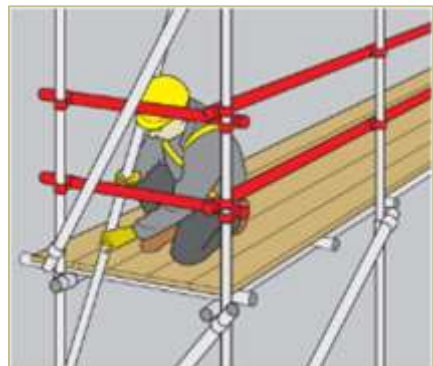
Figure40: Safe handling bay (with double guardrails, stop end returns) - used for raising and lowering materials.
