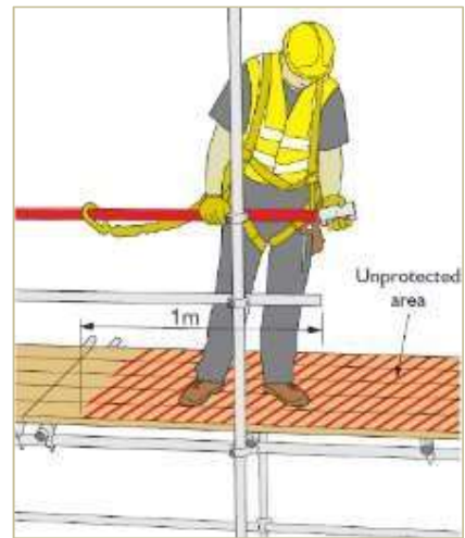
Figure 37: Scaffolders working without a fully-boarded platform
