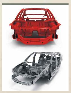
The survey reveals a good correlation between the imperfections in automotive body and the age of the vehicle. Body parts close to the road are most prone to imperfections such as blisters and surface rust. The survey reasonably establishes that the conversion of car body panels manufactured in India from painted cold rolled steel to painted galvanized steel will significantly improve the corrosion performance as was the case in North America.
